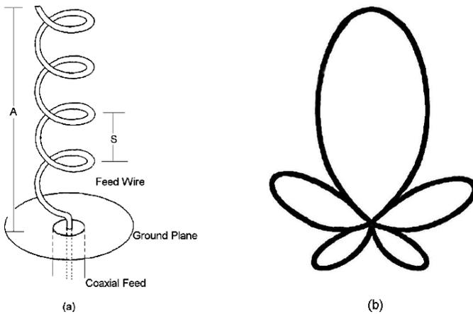
**Figure 4: Helical directional antenna with circular polarization.**<sup>7</sup>
