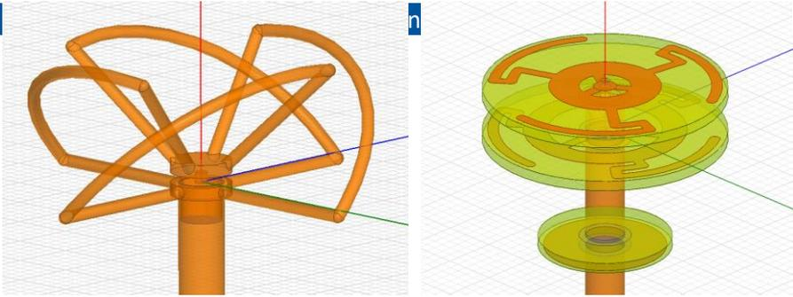
**Figure 3: Designs of non-directional antennas with circular polarization.**<sup>10</sup>
