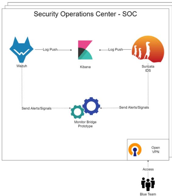
**Figure 5: The Security Operations Center Cyber Range of the Red Ranger and Its Components.**
